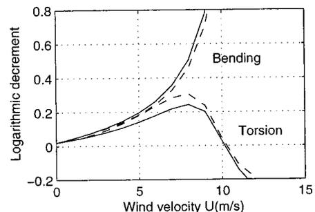
Fig. 2. Damping ratio versus wind velocity (airfoil)
