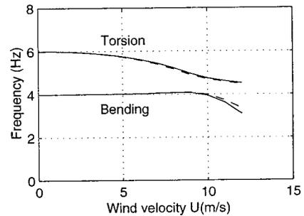
Fig. 1. Frequency versus wind velocity (airfoil)
