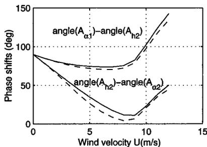
Fig. 4. Phase shifts versus wind velocity (airfoil)
