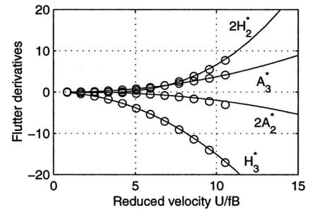
Fig. 6. Comparison of flutter derivatives (twin-box section;—target and *o* identification)
