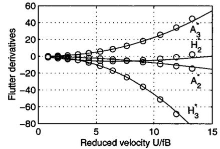
Fig. 5. Comparison of flutter derivatives (airfoil;—target and *o* identification)
