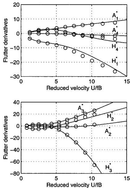
**Fig. 7.** Comparison of flutter derivatives (rectangular section  $B/D = 10$ ;—target and  $\circ$  identification)
