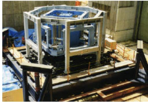
Figure 27. HMD installed in Mitsubishi Heavy Industries Building
