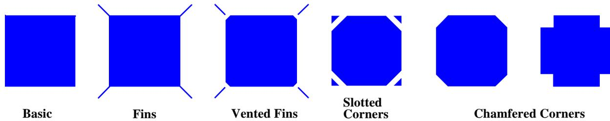
Figure 6: Aerodynamic Modifications to Square Building Shape.
