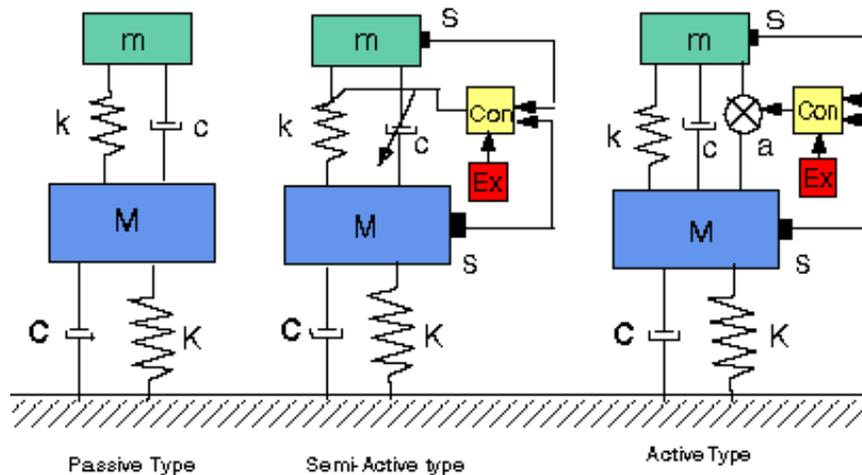
Figure 10: Schematic of various auxiliary damping devices utilizing inertial effects.
