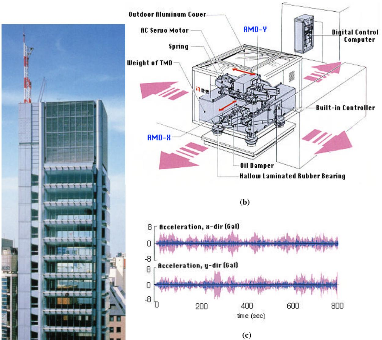
Figure 22: (a) Ando Nishikicho Building; (b) Schematic representation of its hybrid system; (c) performance of system, controlled and uncontrolled (taken from Kajima Corporation)
