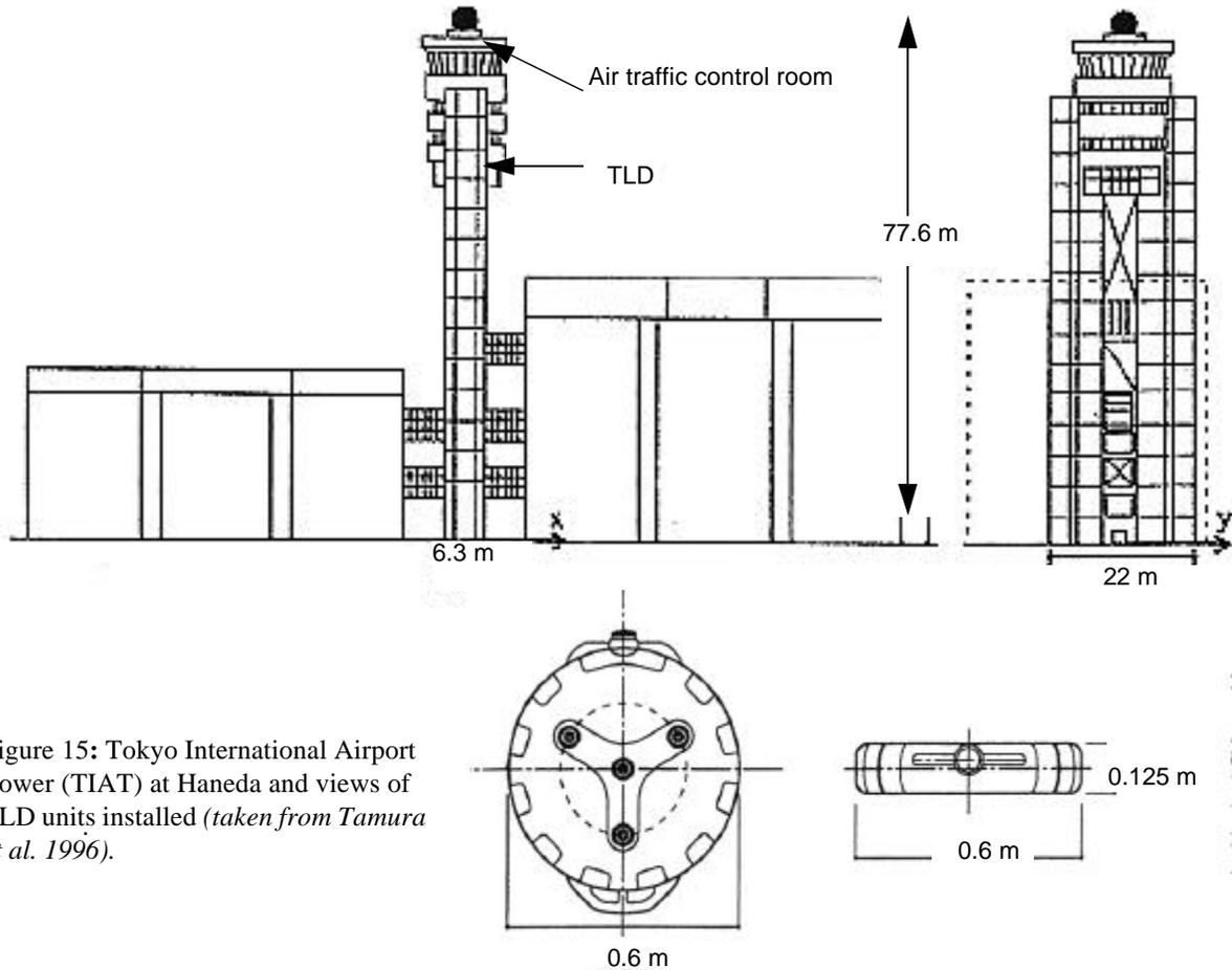
Figure 15: Tokyo International Airport Tower (TIAT) at Haneda and views of TLD units installed (taken from Tamura et al. 1996).
