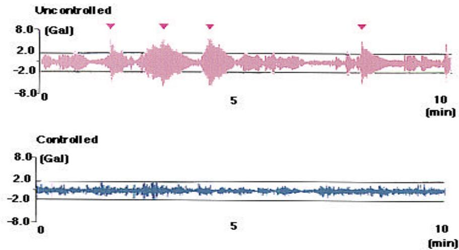
Figure 19: (a) Kyobashi Siewa Building and (b) its AMD unit: (c) performance of structure under wind. (taken from Kajima Corporation).
