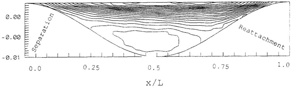
Fig. 4. Streamlines of flow over wavy surface.
