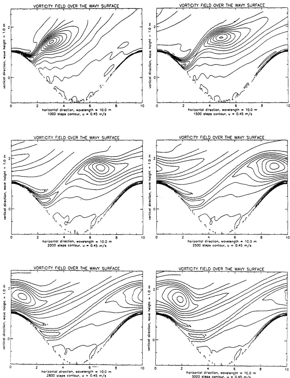
Fig. 3. Vorticity contours of airflow over a sinusoidal boundary at different time steps.
