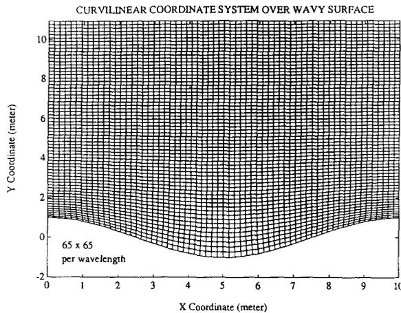
Fig. 1. A curvilinear mesh over a sinusoidal wavy surface.
