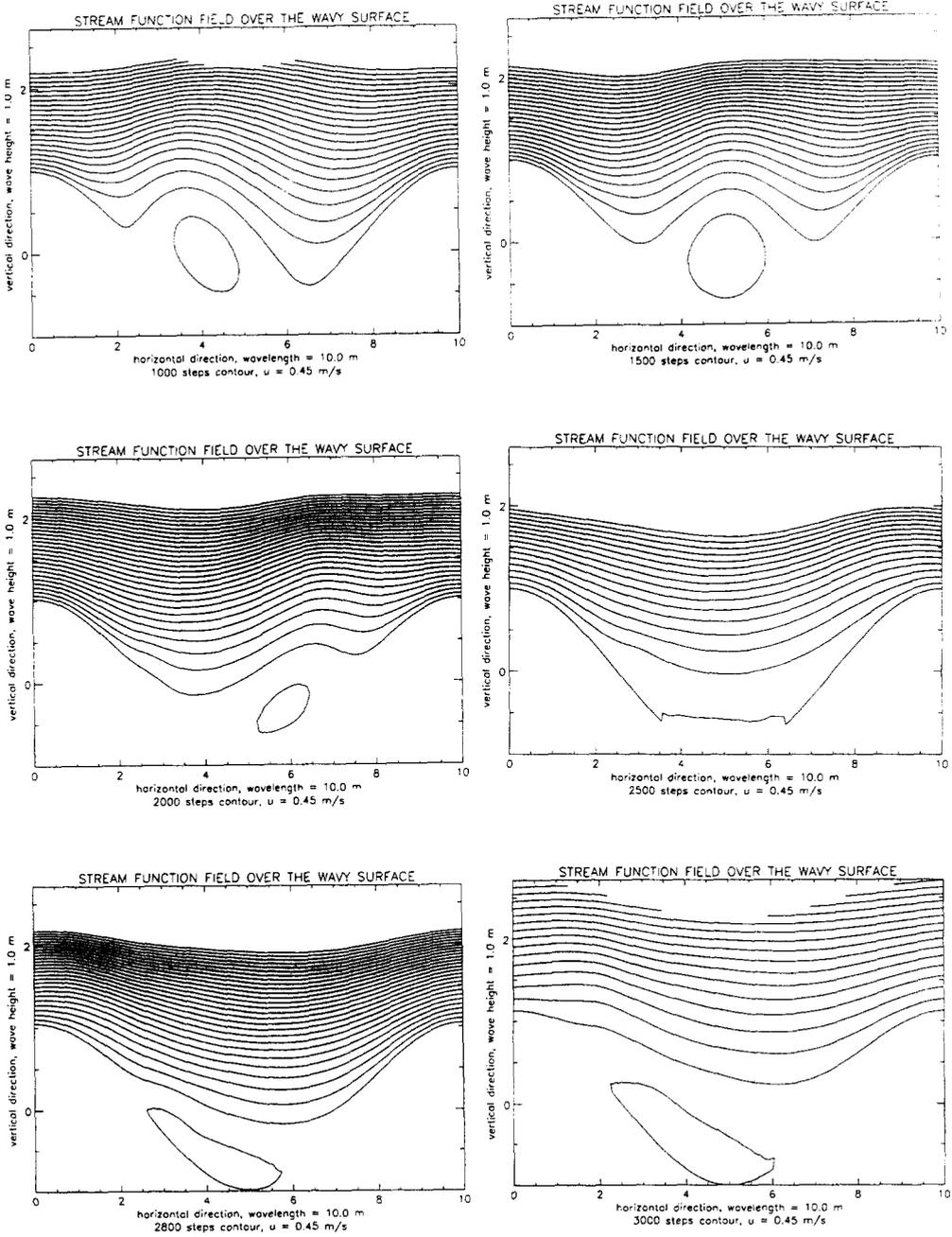
Fig. 2. Streamlines over a sinusoidal wavy surface at different time steps.
