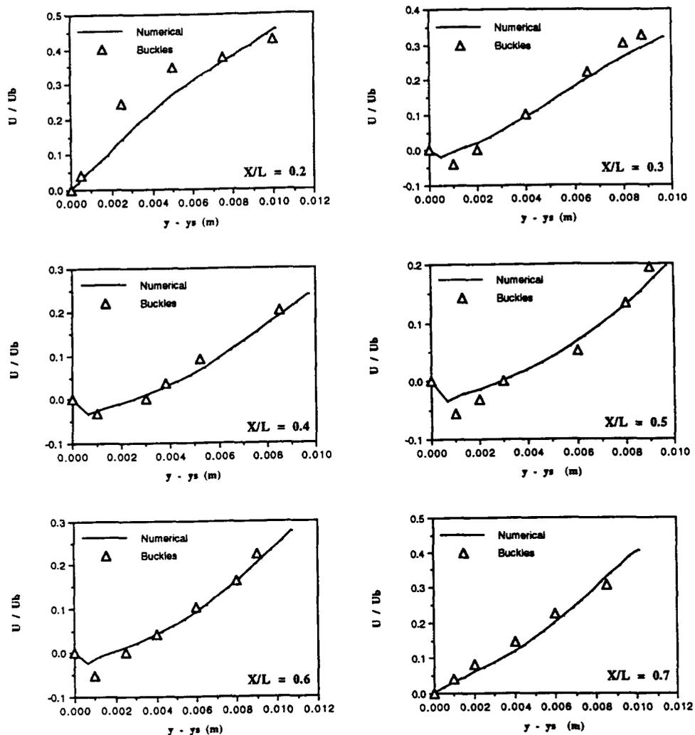
Fig. 5. Comparison of horizontal velocity profiles obtained from numerical and water tunnel experiments.
