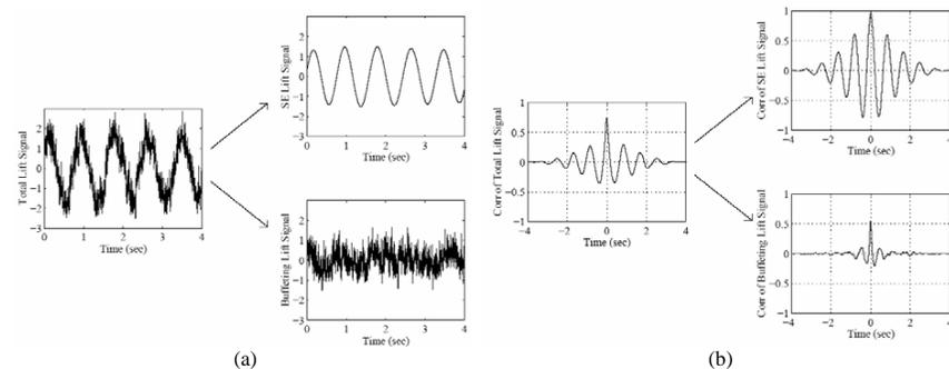
Figure 7: For turbulence case 12b, a reduced velocity of 20 and a spanwise separation of  $1.2B$ : (a) Separation of self-excited and buffeting components of the lift force and (b) an example case for correlation of the lift force.
