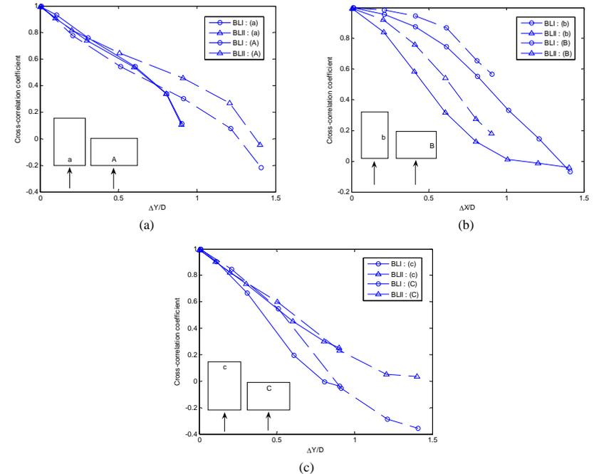
Figure 3: Chordwise cross-correlation structure on the (a) windward, (b) side and (c) leeward surfaces.
