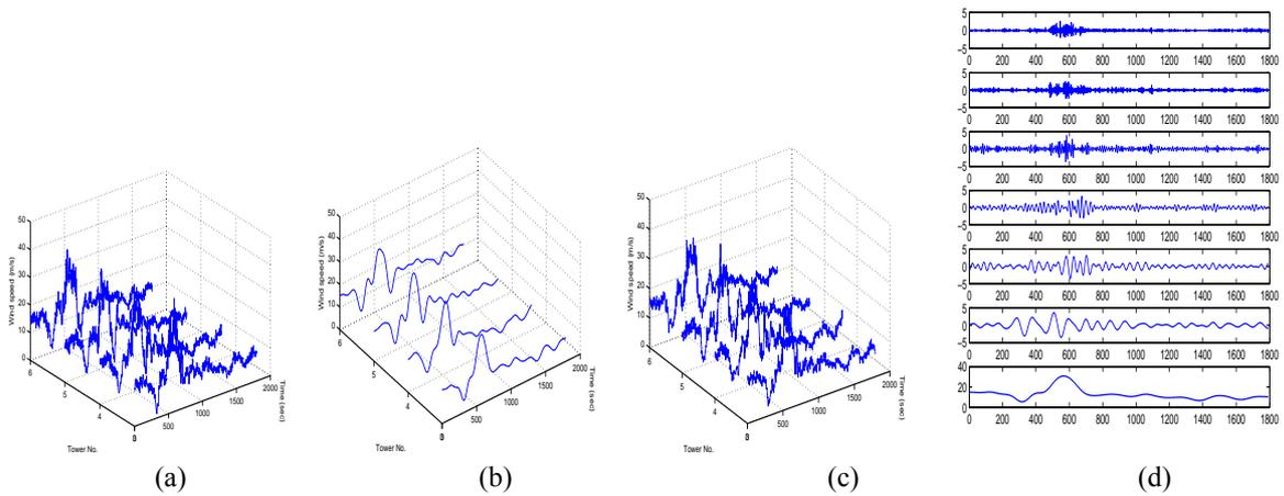
Figure 1: Downburst wind 263 part (a) measurement (b) time-dependent mean (c) simulation (d) decomposition
