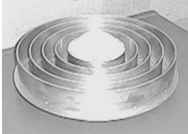
Figure 1: Choke ring antenna used in study.
