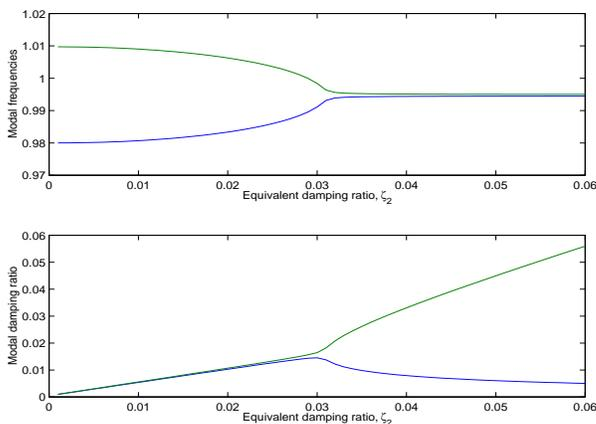
Figure 5. Modal frequencies and damping ratios in the secondary system (liquid damper), the *beat phenomenon* ceases to exist. This is attributed to the coalescing of the modal frequencies of the combined system to a common frequency over that range of damping in the secondary system.
